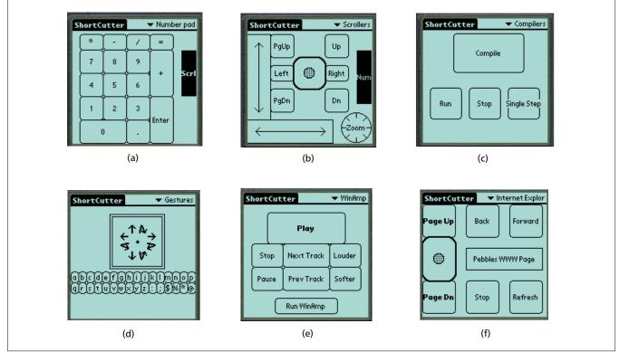
**Figure 3.** Panels created with Shortcutter: (a) a numeric keypad; (b) a collection of scrollers and a knob; (c) buttons for controlling any of a set of compilers; (d) a gesture pad and two rows of small buttons; (e) a controller for the WinAmp MP3 player for PCs; and (f) a panel for browsing in Internet Explorer.
