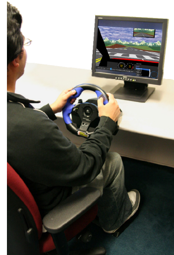
Figure 1. The first author performing input on a small touchpad with his right thumb during simulated driving. The touchpad is mounted in the surface of the wheel at the 2 o'clock position.
