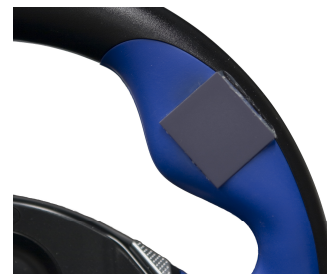
Figure 2. The Synaptics StampPad embedded flush with the surface of a Logitech Driving Force steering wheel.
