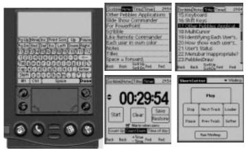
**Figure 1.** At the left is the Remote Commander's keyboard on a Palm Pilot for controlling a PC. At top right are the notes, titles, and timer panels of the Slide Show Commander program. At the bottom right is a panel created with Shortcutter to control the WinAmp music program which runs on a PC.
