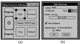
**Figure 6.** (a) The editing mode of Shortcutter with the Back button selected. (b) Setting the properties of the Back button so when you click on the Back button at run-time, it sends to the PC the keystroke Alt-left-arrow.
