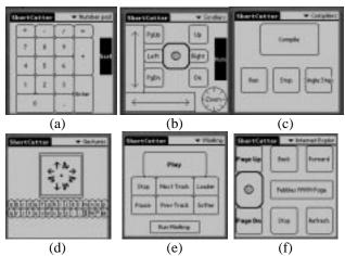
**Figure 5.** Panels created with Shortcutter. (a) A numeric keypad, (b) a collection of scrollers and a knob, (c) buttons for controlling any of a set of compilers, (d) a gesture pad and two rows of small buttons, (e) a controller for the WinAmp PC program, and (f) a panel for browsing in Internet Explorer.
