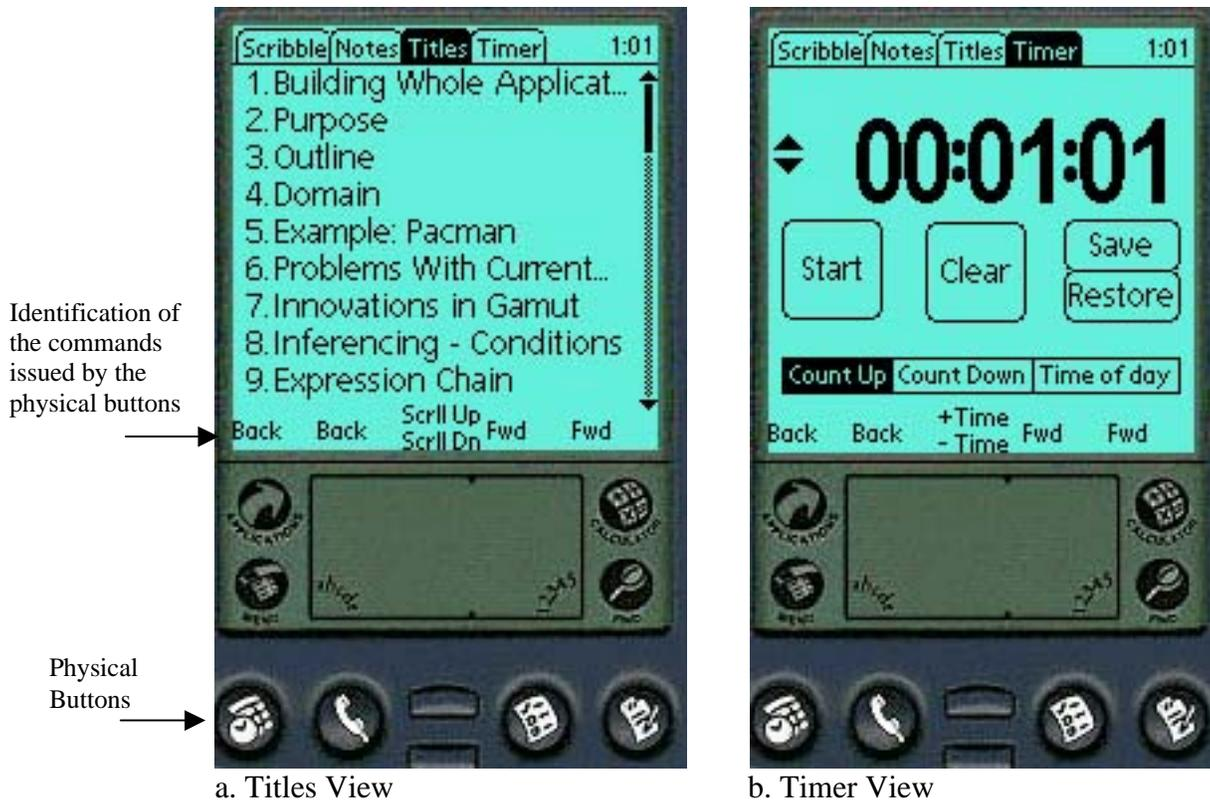
Figure 3. Design Changes in SlideShow Commander 3.0. (a) Addition of user-defined hard button commands for basic slide navigation controls; (b) Addition of a timer to the application.
