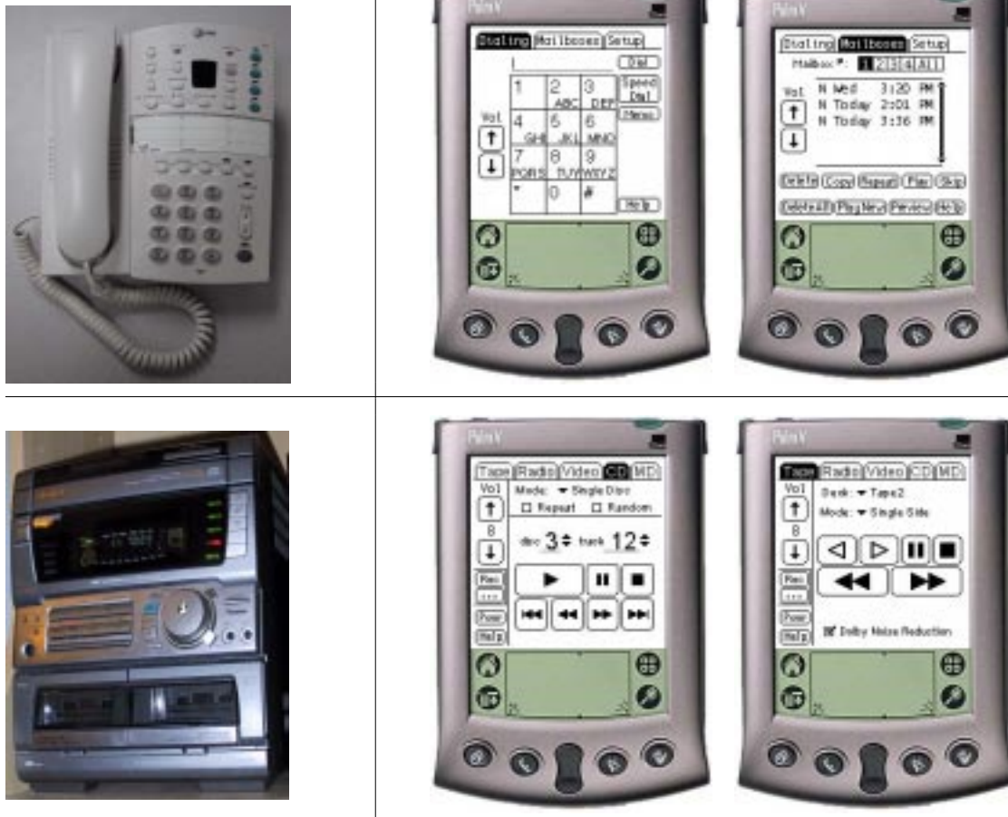
Figure 1. The actual devices (left) and some hand-drawn control panels for the Palm for the AT&T phone (top) and AIWA stereo (bottom).
