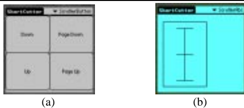
Figure 4. (a) The revised button scroller on the WorkPad used in the second experiment. (b) The “absolute scroller”.
