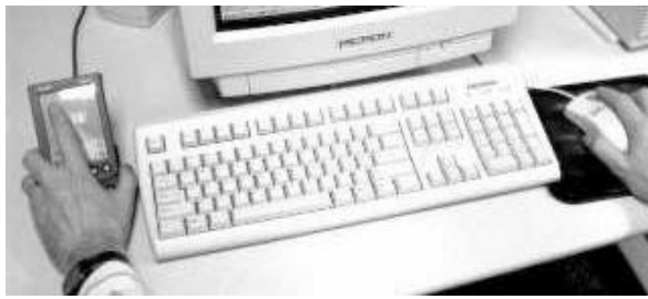
Figure 1. Typical configuration, with a PDA in its cradle on the left of the keyboard, and the user's hands on the PDA and the mouse.
